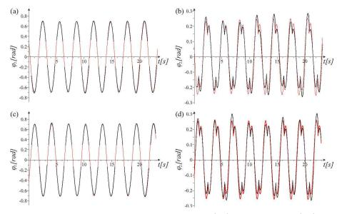
**Fig. 2.** Comparison between time traces of the bell (a,c) and the clapper (b,c) obtained numerically (red lines) and experimentally (black dots). Subplots (a,b) correspond to the data obtained from the first recording and (c,d) from the second one.
