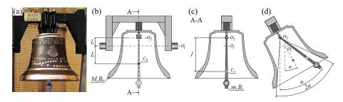
**Fig. 1.** *"The Heart of Lodz"* the biggest bell in the Cathedral Basilica of St Stanislaus Kostka (a) and it's schematic model (b,c,d) along with physical and geometrical quantities involved in the mathematical model of the system.
