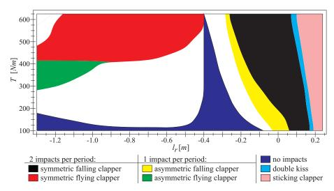
**Fig. 5.** Two parameter ringing schemes diagram showing the behavior of the system for different values of  $l_{\tau}$  and T.
