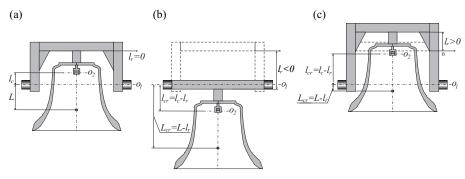
**Fig. 3.** Description of parameter  $l_r$ : (a) reference yoke design  $l_r = 0$ , (b)  $l_r < 0$ , (c)  $l_r > 0$ .
