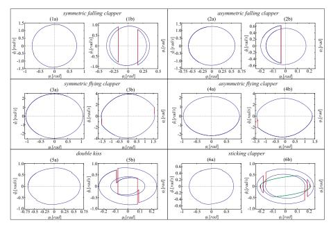
**Fig. 4.** Presentation of the most common working schemes of church bells. Subplots (a) and (b) present phase portraits of the bell and the clapper respectively.
