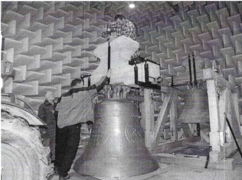
Fig. 2: Bells being set up for ringing tests in the laboratory
