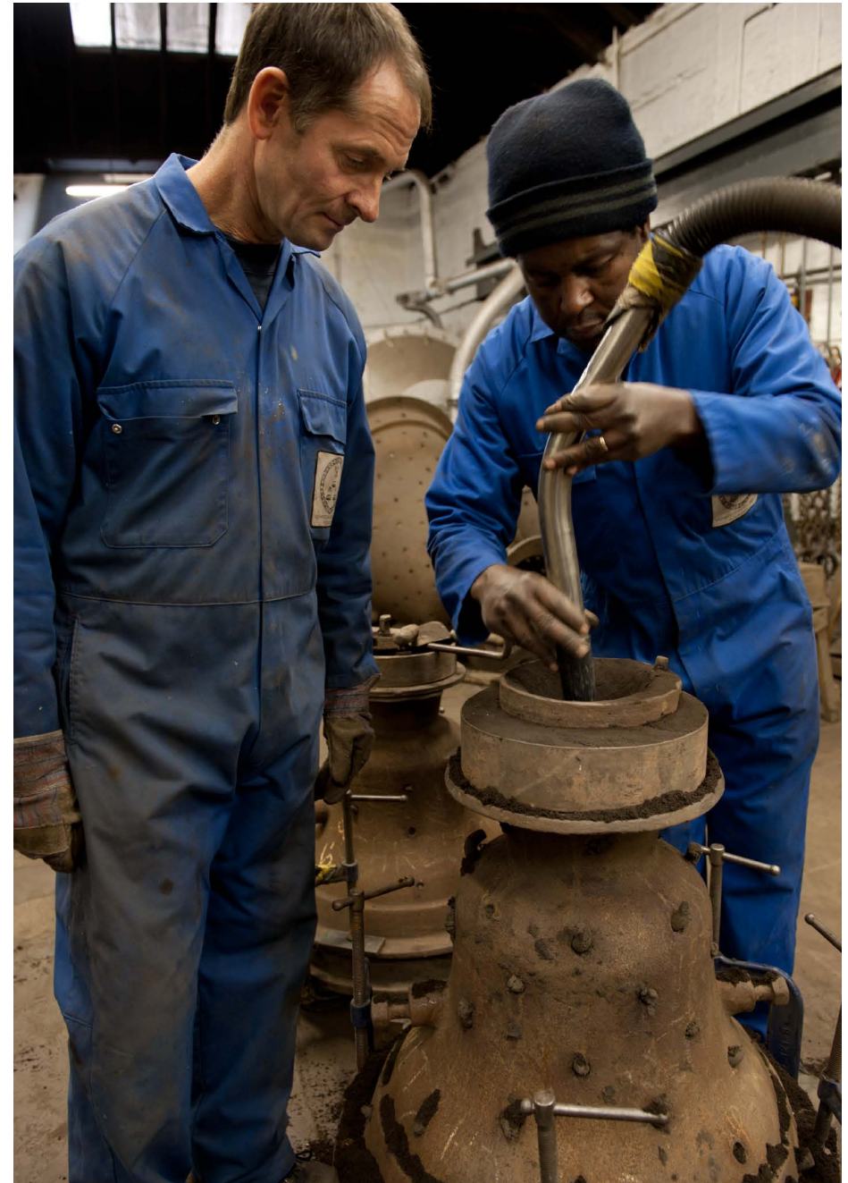
Preparing a bell flask in 2011 (photograph by Derek Kendall, © Historic England Archive)
